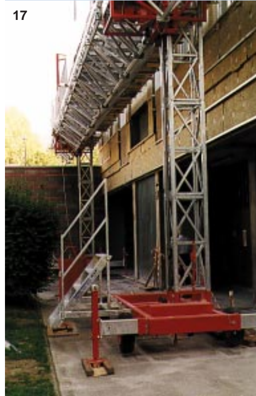
ELECTROSCAF 3000 working platform with a single or double mast • maximum height: 150 m • max. load (evenly spread): 1200 or 3000 kg • maximum length of platform: 10 or 24 m
