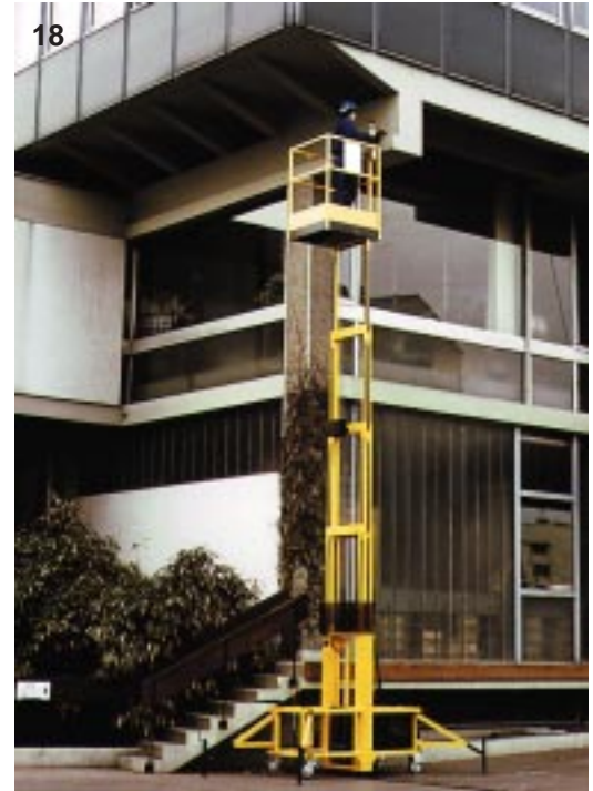
TRACTELIFT mobile work platform • max. height of the floor panel 7.3 m to 10.3 m (according to the model) • maximum load: 225 kg • power supply by rechargeable battery • standard model with swivel wheels • towable model (optional)
